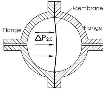
**Figure 4.** A cutaway view of the DC flow suppresser.
