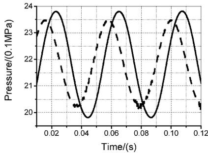
**Figure 5.** Two typical pressure waves when the system reached the energy balance. The solid line and dashed line present the pressure wave at the inlet of the PTC and in the TE near the main water-cooled heat exchanger, respectively.
