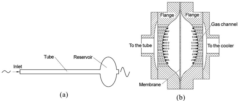
**Figure 2.** (a) A schematic diagram of an acoustic amplifier composed of a tube and a reservoir; (b) A cutaway view of the reservoir with a membrane.
