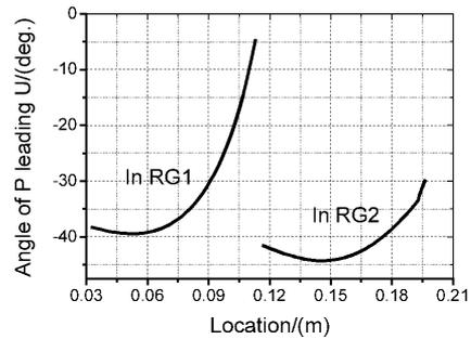
**Figure 6.** The distribution of angle pressure leading volume flow in the regenerators.
