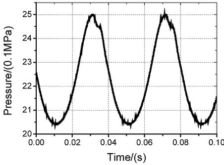
**Figure 3.** A typical pressure waveform with the crest distorted.
