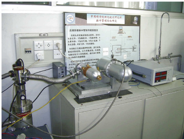
Figure 2. PTC test facility, it allows the operation of various inclination angles.
