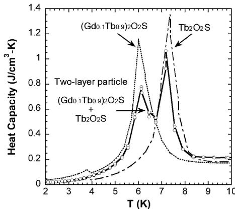
**Figure 4.** Experimental results on the heat capacity for  $(Gd_{0.1}Tb_{0.9})_2O_2S$ ,  $Tb_2O_2S$  and two-layer  $(Gd_{0.1}Tb_{0.9})_2O_2S + Tb_2O_2S$  regenerator particles.
