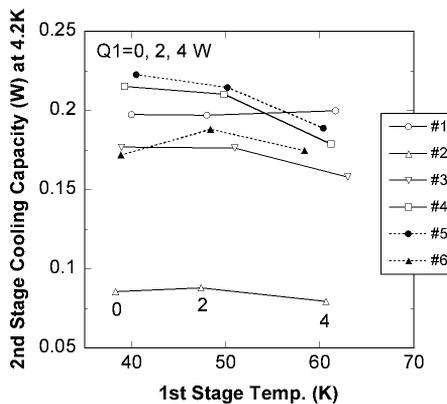
**Figure 7.** Experimental results for 2nd-stage cooling capacity at 4.2 K for the 0.1 W GM cryocooler as a function of 2nd-stage-regenerator configuration and 1st-stage temperature.
