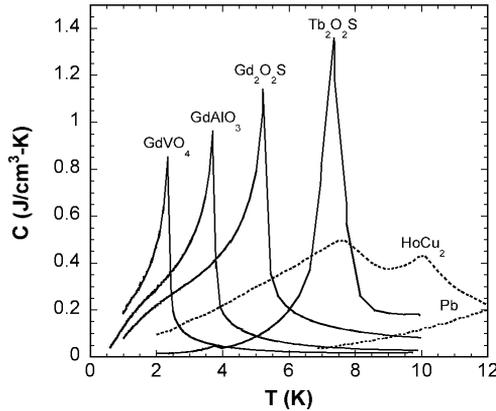
**Figure 1.** Heat capacity data at zero magnetic field for the oxide magnetic materials  $\text{GdVO}_4$ ,  $\text{GdAlO}_3$ ,  $\text{Gd}_2\text{O}_2\text{S}$  and  $\text{Tb}_2\text{O}_2\text{S}$ ; also shown are Pb and  $\text{HoCu}_2$ .
