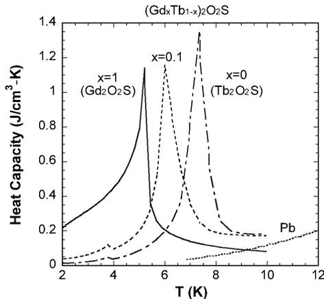
**Figure 2.** Volumetric heat capacity of the  $(\text{Gd}_x\text{Tb}_{1-x})_2\text{O}_2\text{S}$  system.
