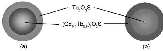
**Figure 3.** Structure of two-layer magnetic regenerator material. The particle consists of  $Tb_2O_2S$  and  $(Gd_{0.1}Tb_{0.9})_2O_2S$  for inner and outer layer in case (a), or outer and inner layer in case (b), respectively.
