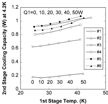
**Figure 5.** Experimental results for 2nd-stage cooling capacity at 4.2 K for the 1W GM cryocooler as a function of 2nd-stage-regenerator configuration and 1st-stage temperature.
