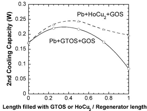
**Figure 8.** Experimental results on the cooling capacity of 2nd stage regenerator at 4.2 K for the 1st stage temperature for 0.1 W GM cryocooler.
