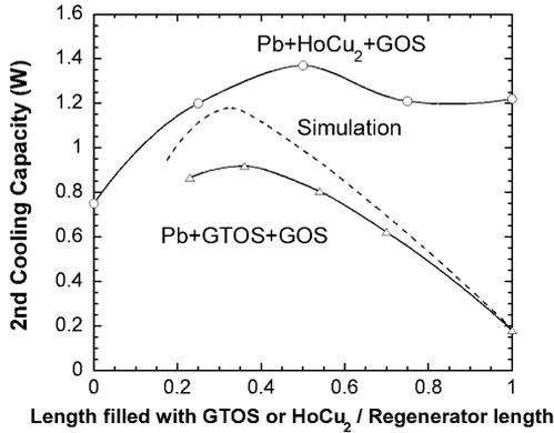
**Figure 6.** Experimental results for the cooling capacity of the 2nd stage at 4.2 K as a function of the fraction of the second-stage regenerator length filled with  $\text{HoCu}_2 + \text{GOS}$  or  $\text{GTOS} + \text{GOS}$ .
