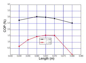
Figure 1. COP as function of length of regenerator for fixed frequency, area, PV1, hot end temperature (f=50 Hz, PV1=1 W,  $T_{\mu}$ =100 K, D=8.9 mm)
