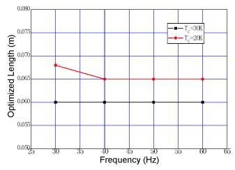
Figure 2. Optimized length of regenerator as function of frequency. (PV1=1 W,  $T_{H} = 100 \text{ K}$ , D=8.9 mm)
