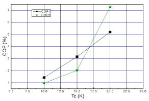
Figure 6. COP as function of cold end temperature for fixed volume rate of cold end. ( $T_{H}$ =80 K, L=60 mm, D=8.9 mm)
