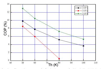
Figure 4. COP as function of hot end temperature for fixed volume rate of cold end. (T =20 K, L=60 mm, D=8.9 mm)
