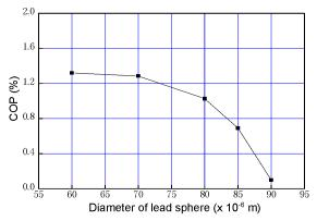
Figure 8. COP as function of diameter of lead sphere for fixed mass rate of cold end. ( $T_{H}$ =80 K, Tc=10 K, L=60 mm, D=8.9 mm)
