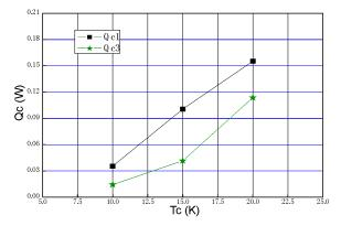
Figure 5. Net refrigeration power as function of cold end temperature for fixed volume rate of cold end. ( $T_{\mu}$ =80 K, L=60 mm, D=8.9 mm)
