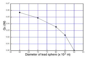
Figure 7. Net refrigeration power as function of diameter of lead sphere for fixed mass rate of cold end. ( $T_{\rm H}$ =80 K, Tc=10 K, L=60 mm, D=8.9 mm)
