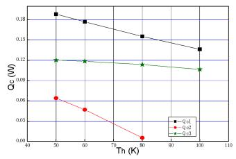
Figure 3. Net refrigeration power as function of hot end temperature. ( $T_c = 20$  K, L=60 mm, D=8.9 mm)
