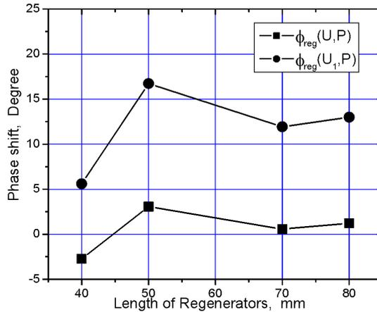
**Figure 11.** Phase shift of different regenerators
