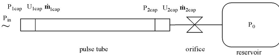
Figure 4. Computed model for phase shift of a capacity element
