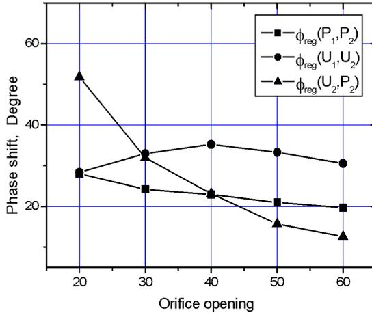
Figure 6. Phase shift depending on orifice opening
