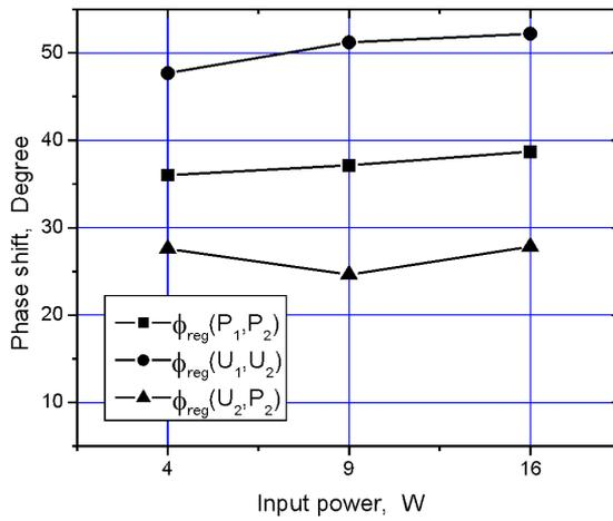
Figure 7. Phase shift depending on input power
