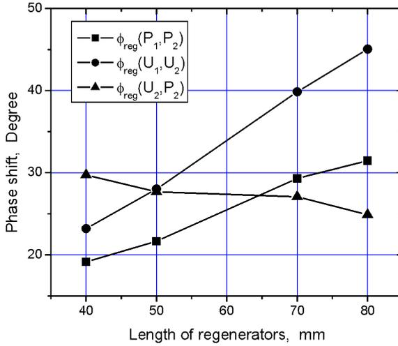
Figure 9. Phase shift depending on length of regenerators
