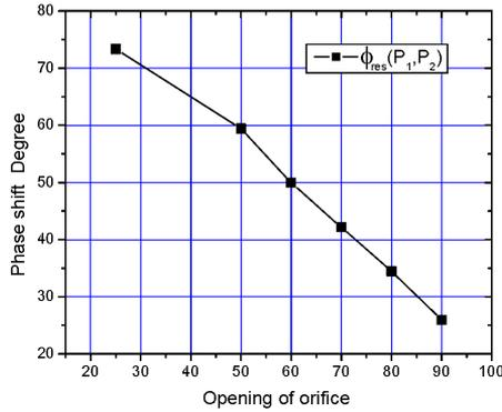
Figure 3. Phase shift of pressures at both sides of a resistance element.
