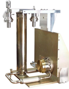
Figure 6. The flight NICMOS Cooling System in preparation for installation on HST.
