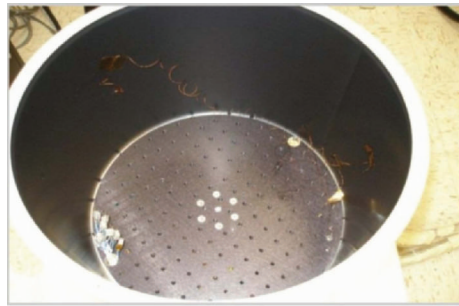
Figure 7. Cold plate for mounting cryocooler
