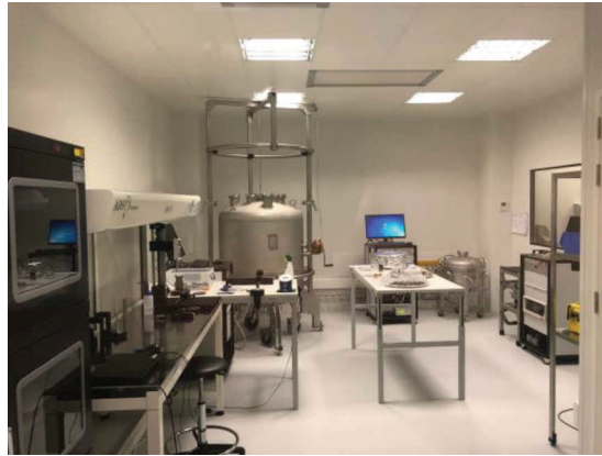
Figure 8. ISO8 clean room with test TVAC test benches and ISO5 assembling hoods at Absolut System
