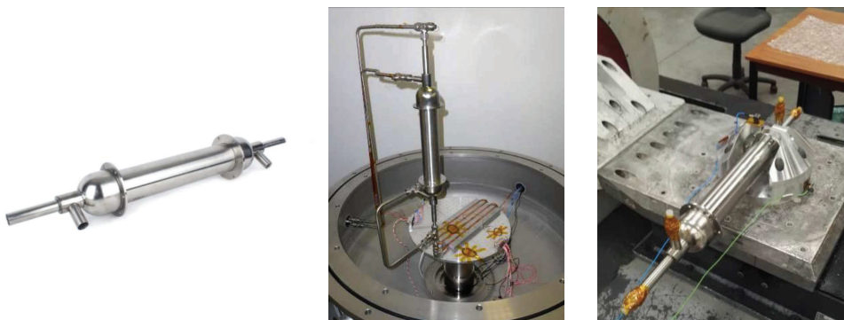
Figure 4. Picture of the recuperator prototype, test setup in vacuum test chamber and shaker
