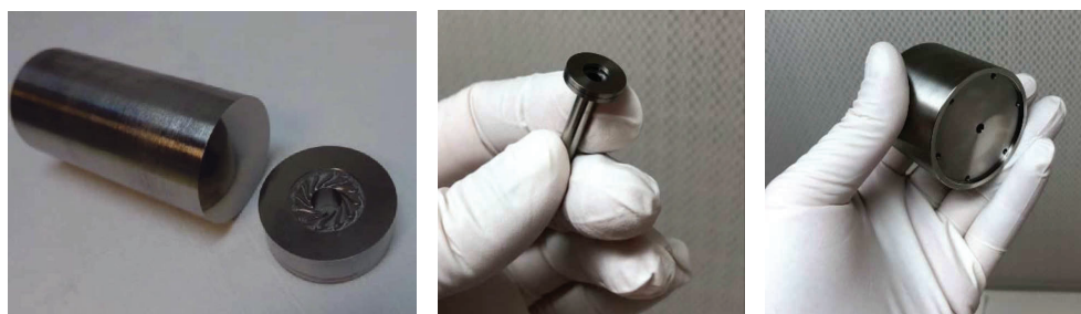
Figure 6. Cryogenic expander: impeller before diffusion welding, final shaft, expander assembly without the rotor
