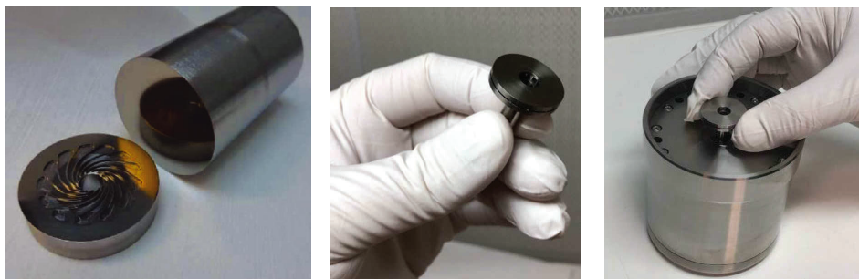
Figure 5. Centrifugal compressor: impeller before diffusion welding, final shaft, compressor assembly with the rotor
