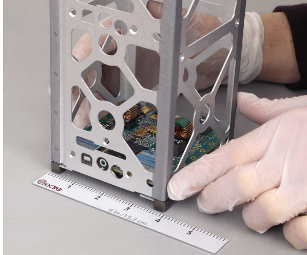
Figure 10. MCCE-TS During Integration with CubeSat Frame. The MCCE-TS is a single board assembly designed to fit on a side of a 1U CubeSat.
