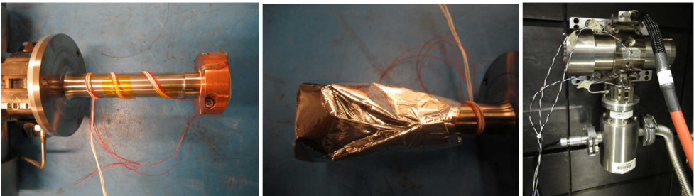
Figure 3. Wiring and instrumentation (left), radiation insulation (middle) and mounting inside climate chamber (right).
