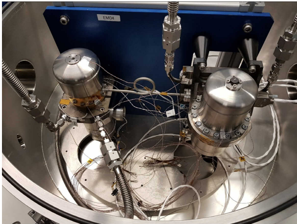
Figure 4. The LPTC EM04 – inside the Cryocooler Performance Characterization Facility in a non-intercepted configuration.
