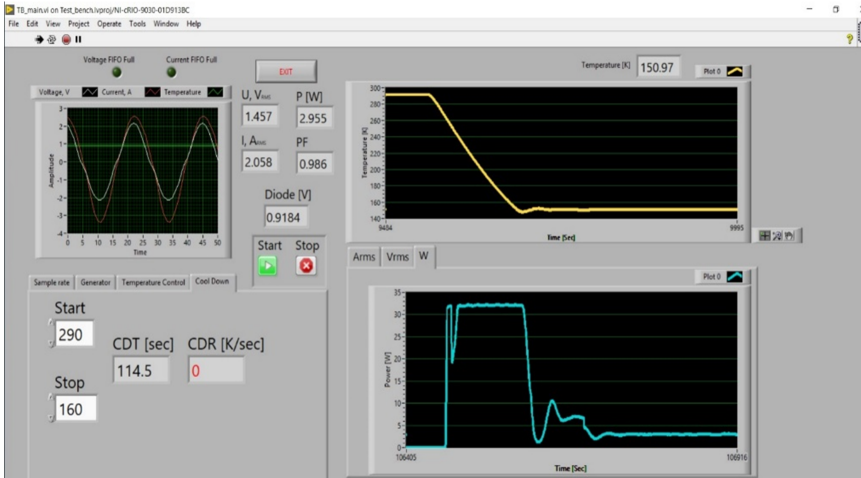
Figure 8. Cooldown from 300 K to 160 K
