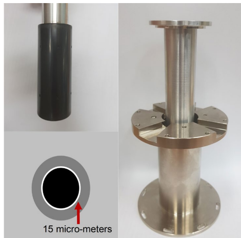
Figure 4. Photo of piston-cylinder assembly showing radial gap clearance
