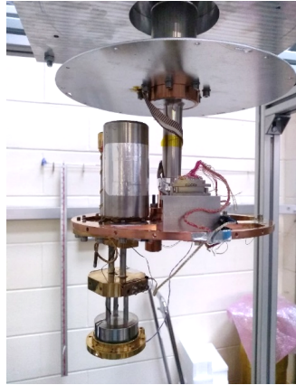
Figure 2. GL4 module interfaced to the GM cold head.
