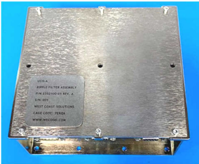
Figure 4. UCIS IRF. Measured results: >90\% above 25W, peak efficiency 97.2% at 151W.
