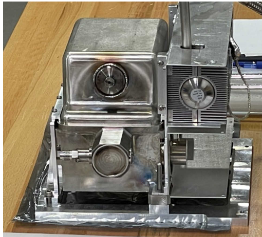
Figure 8. In-process assembly photograph of cryocooler risk reduction subsystem. Photograph taken after cold heat instrumentation and vacuum integration, during purge-charge, and before final duct close out.
