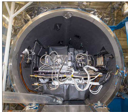
TIRS II TVAC Testing
