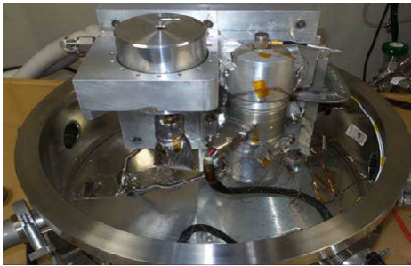
Figure 2. MCP mounted in the test fixture, instrumented for thermal performance test
