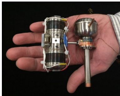
Figure 3. Lockheed Martin micro pulse tube cryocooler
