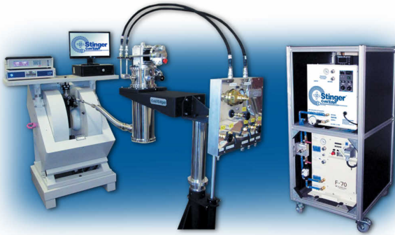
Figure 13. ColdEdge Technologies Stinger® system with SHI cold head
