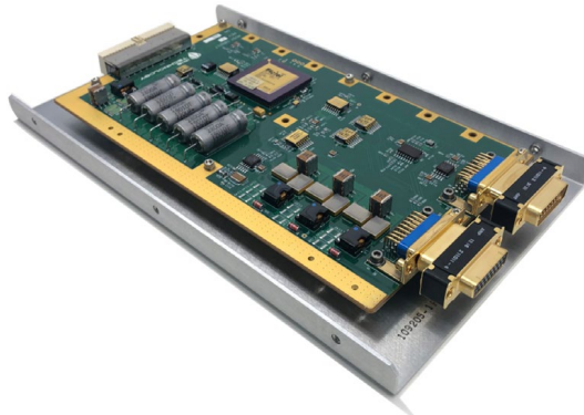
Figure 6. The fully assembled MASPEX Cryocooler Electronics Board (MCEB).
