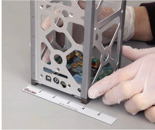
Figure 1. The MCCETS is a single board assembly designed to fit on a side of a 1U CubeSat.
